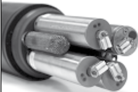
YSI sonde with copper-alloy sensors, wipers, and screens was deployed in the Arabian Gulf for 3 months without maintenance. Copper has chemical properties that deter biofouling from adhering and growing on the sonde's surfaces.
