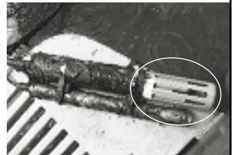
Anti-fouling copper sensors and sonde guard on YSI sonde deployed for more than 1 month without biofouling build-up. Photo: Stephanie Hess, King County, WA.
